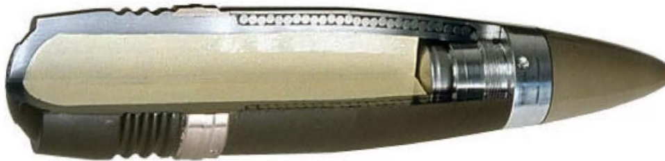
Cutaway of the 40mm 3P shell. The sophisticated fuse and sensors are in the nose. Note the 1,100 pre-fragmented tungsten pellets that surround the 120g PBX charge. When detonated, these are sprayed outward in a lethal cloud of metal that can destroy the delicate systems of missiles or aircraft or take out small boats and personnel. (Image: BAE Systems).
