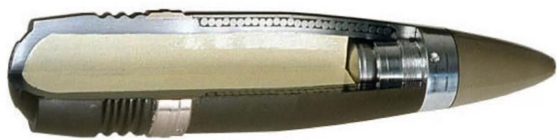
Cutaway of the 40mm 3P shell. The sophisticated fuse and sensors are in the nose. Note the 1,100 pre-fragmented tungsten pellets that surround the 120g PBX charge. When detonated, these are sprayed outward in a lethal cloud of metal that can destroy the delicate systems of missiles or aircraft or take out small boats and personnel. (Image: BAE Systems).
